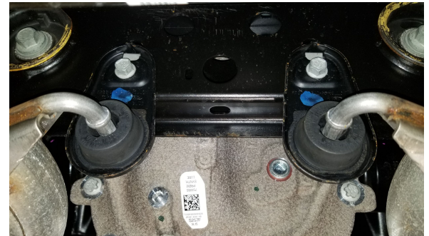
Detail 5: Rear subframe hangers
