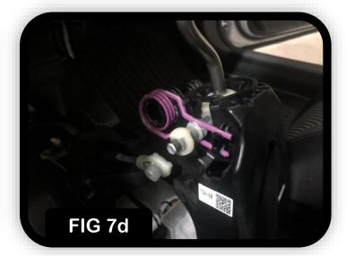
STEP 8 - Re-install Rocker and Connect Gate Change Cable
